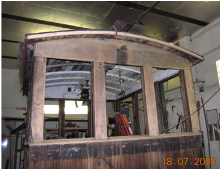
No. 2 cab end with new arch. Stripped and ready for priming.
