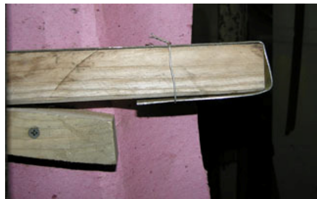
Tension straps around end of arch wood.
