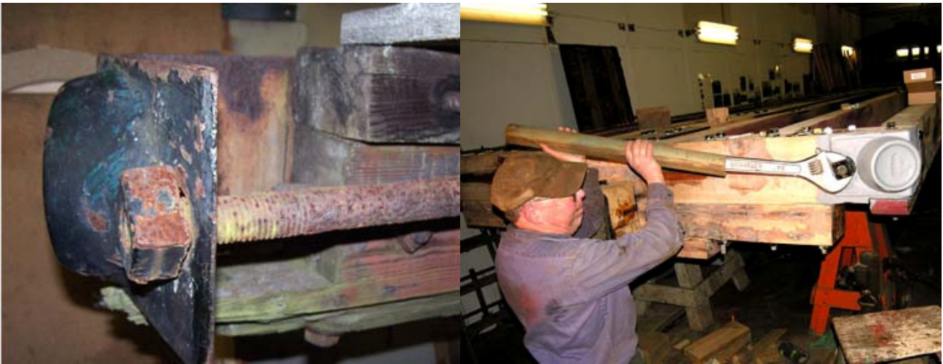
Truss rod ends before and after.
