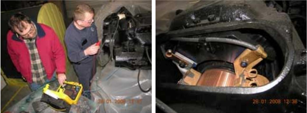
Randy Leclair monitoring the new AEMC 1060 megohmmeter while Roger Paradie makes the connection to the overhauled GE 80 motor at A. C. Electric
