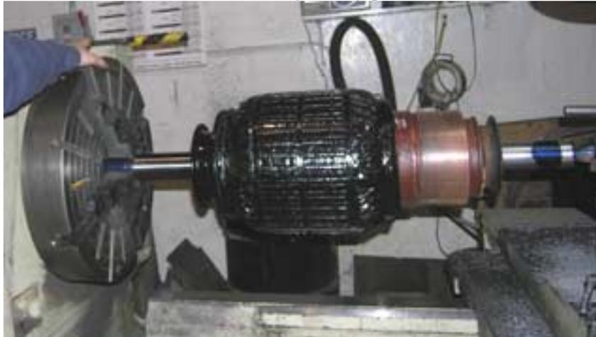
Armature in the lathe for truing the shaft.
