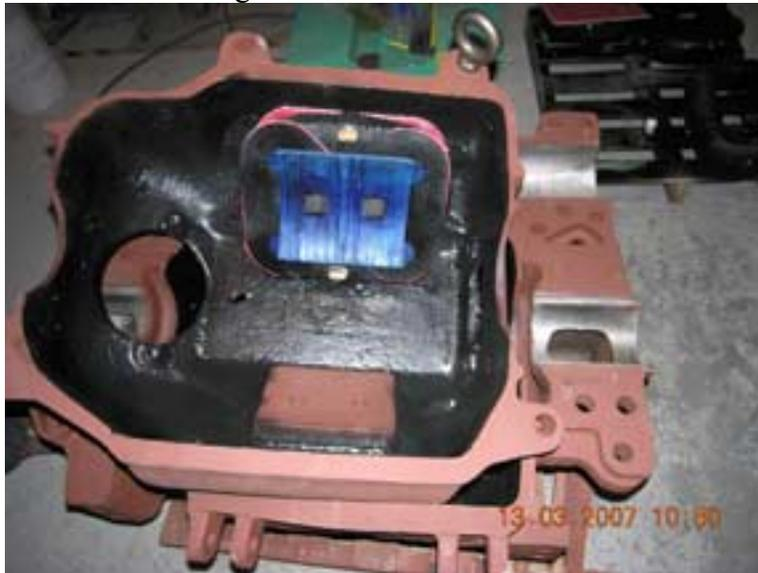
Case with first field coil installed
