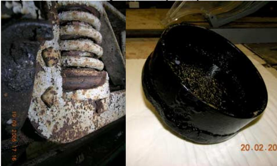
Original cracked spring cup and rebuilt and repainted<sup>2</sup> one.
