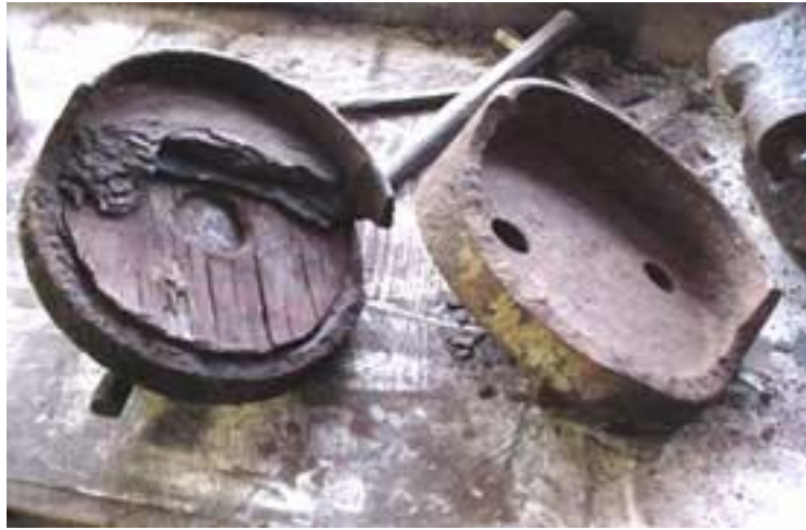
Equalizer spring cups before and after removing rust build-up. Note oak disc under the rust.
